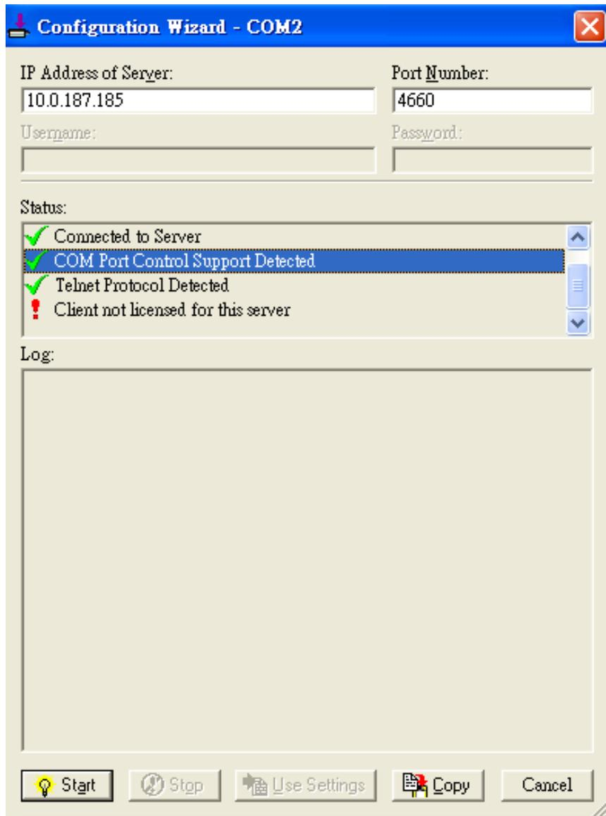
Figure 6.13 Licensing Issue of Serial/IP Utility Software
