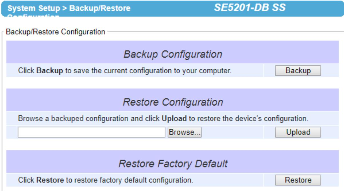
Figure 4.37 Backup/Restore Settings Web Page under System Setup
