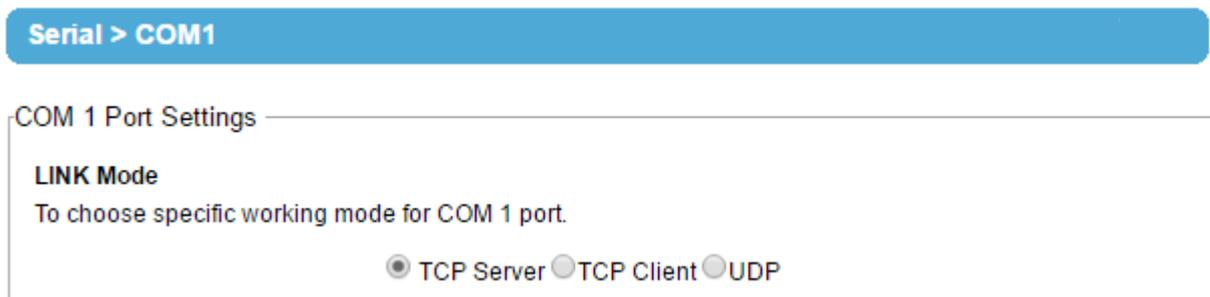
Figure 5.1 Link Mode Options for COM1 Port
